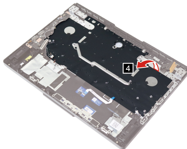
Figure 34. Peel back the protective mylar
