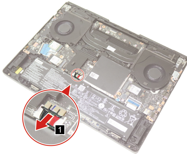
Figure 8. Disconnect the battery pack cable
